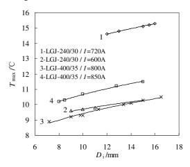
Figure 3 The relationship between the maximum temperature of conductor  $T_{\text{max}}$  and the thickness of ice  $D_{\text{i}}$ Figure 3 shows that  $T_{\text{max}}$  increases with increasing  $D_{\text{i}}$ , and
