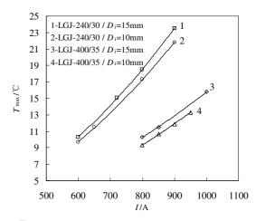
Figure 4 The relationship between the maximum temperature of conductor  $T_{\text{max}}$  and ice-melting current *I*
